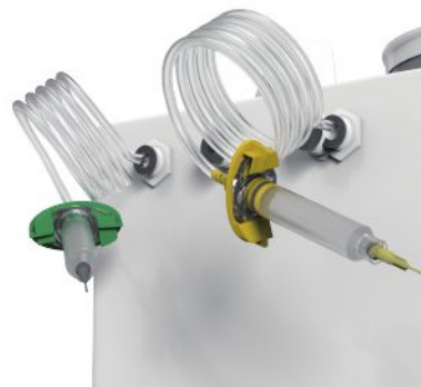
Blow to remove dust (green), suction to remove clogs (yellow)
