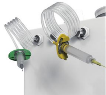
Blow to remove dust (green), suction to remove dirt/wax (yellow)
